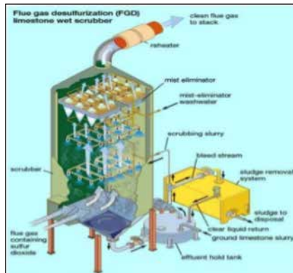
Pic 5.5: FGD system
