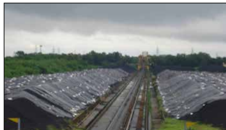
Pic 2.12: Covered coal piles
