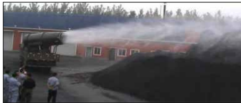
Pic 2.13: Water spraying over piles
